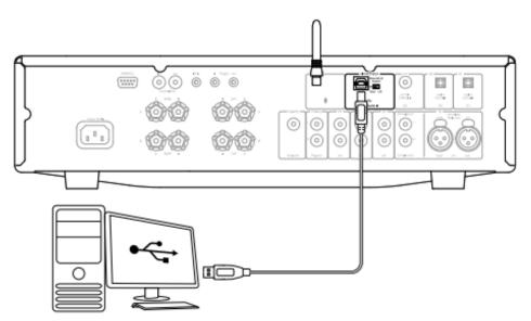
**Important Note:** Always turn the volume to minimum, switch to another input or turn the CXA off before plugging/unplugging cables to the USB input or whilst booting up/shutting down your PC/Mac.
