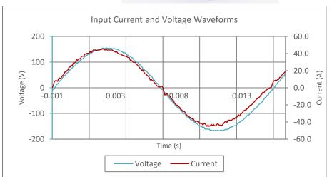
Input AC Current Waveform (ITHD = 3.21%, 50% Load)
