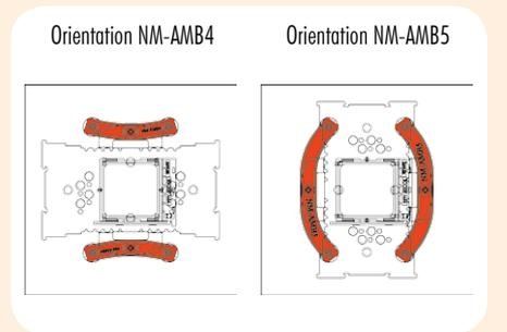
First put the plastic spacers onto the screw threads of the backplate, then fix the mounting bars using the four long screws.
