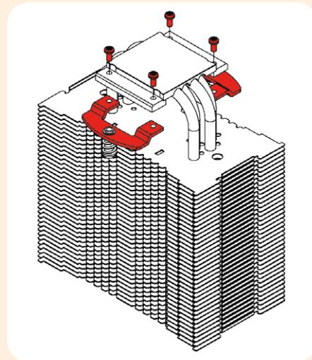
Then fix the new NM-SFB2 fastening brackets to the cooler (you can either use the original screws or the supplied NM-SSC1 screws). Tighten the screws until they stop, but don't use excessive force (max. torque 0.5 Nm).
