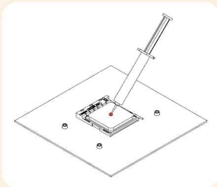
**Caution:** Applying too much thermal paste will lower heat conductivity and cooling performance!
