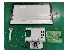
LCD module(together with their casing) is only left after all other parts like electronic units and casing have been removed.
