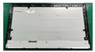
disaaemble screw 7EA and disassemble the PCB
