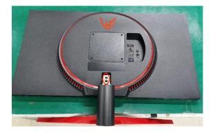
disassemble the latches of three edges
