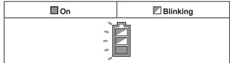
When the tool is overheated, the tool stops automatically, and the battery indicator blinks about 60 seconds. In this situation, let the tool cool down before turning the tool on again.
