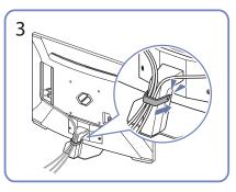
Put both cables in the cable holder on the stand (HOLDER-STAND CABLE) to organise the cables, as shown in the figure.
