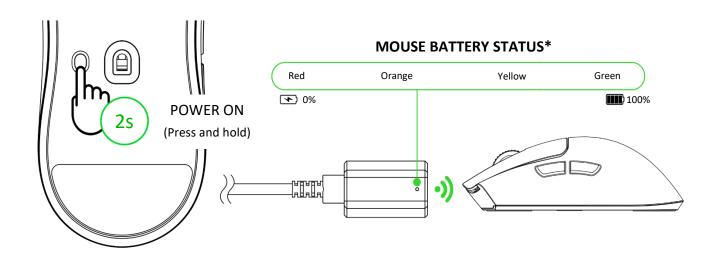
\*Indicator display can be customized to show connection status, mouse battery status (default), or low-battery warning only using the Razer Synapse app.
