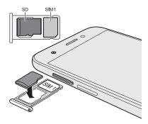
5. When reinserting the tray, make sure it is facing up so that your cards don't fall out. With the outer card holder between your fingers, steadily slide the tray all the way into the slot.
