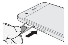
**6.** Make sure the tray is fully inserted and doesn't protrude from the slot.
