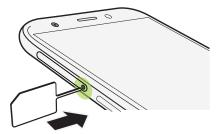
When inserting the eject tool into the tray eject hole to remove the card tray, do not obstruct the tray to avoid damaging the eject mechanism inside the slot.
