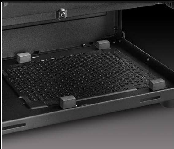
Decoupled Power Supply Mounting
