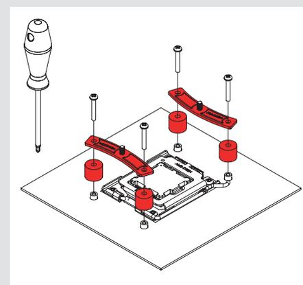
Make sure that the curved sides of the mounting bars are pointing inwards.
