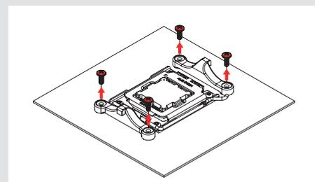
The SecuFirm2™ mounting system will install directly to the stock backplate, so please keep it in place.
