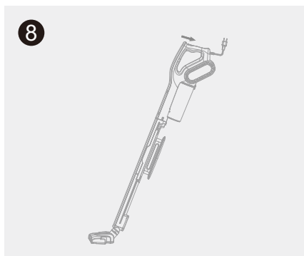
8. Slide the ON/OFF switch to turn the vacuum off and unplug the power cord after using.
