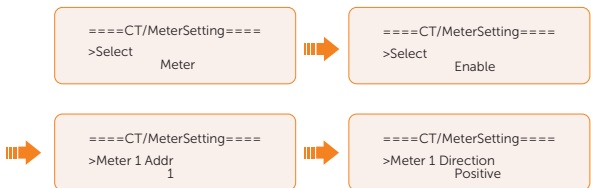
Figure 14-13 Setting meter for the inverter
