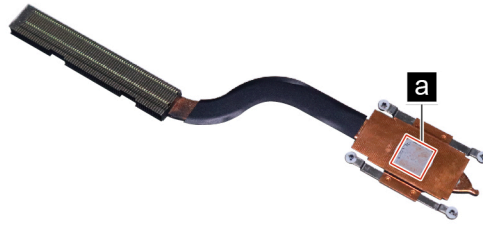
Figure 8. Area(s) on the heat sink where thermal interface materials should be applied
