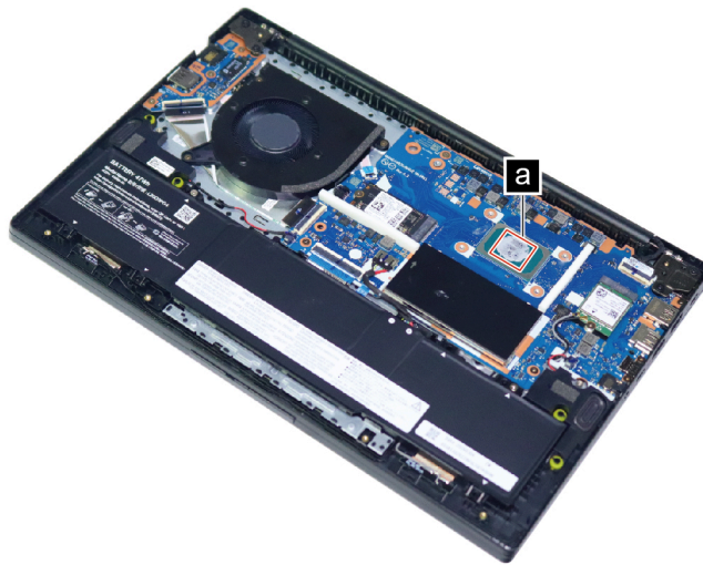
Figure 9. Area(s) on the system board where thermal interface materials are applied
