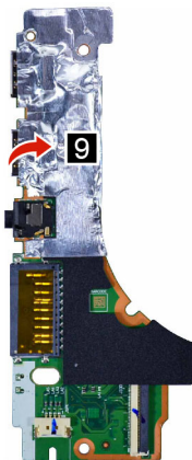
Figure 21. Remove the I/O board mylar
