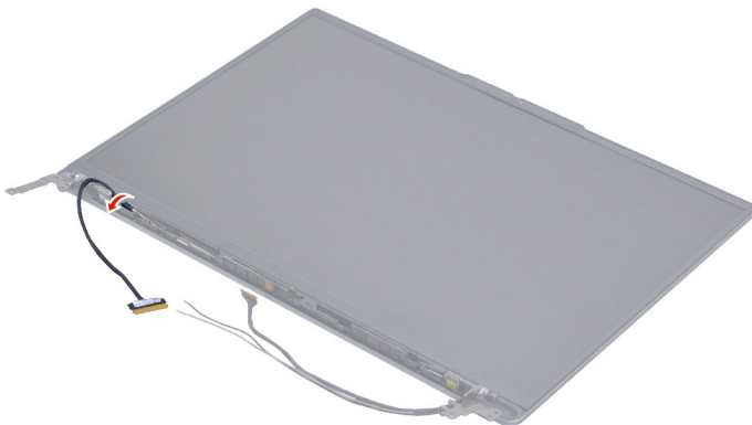
Figure 29. Release the EDP cable
