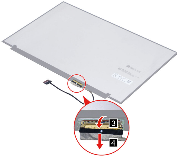
Figure 32. Remove the EDP cable
