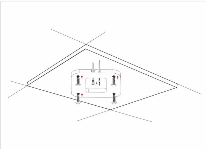
**Step 6** Connect the Ethernet cable to the RJ45 port. If you use a DC adapter to supply power to the AP, connect the power cable to the power jack of the AP.
