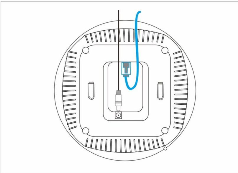
**Step 7** Insert the hooks of the AP inside the slots of the mounting bracket to fix the AP onto the mounting bracket.
