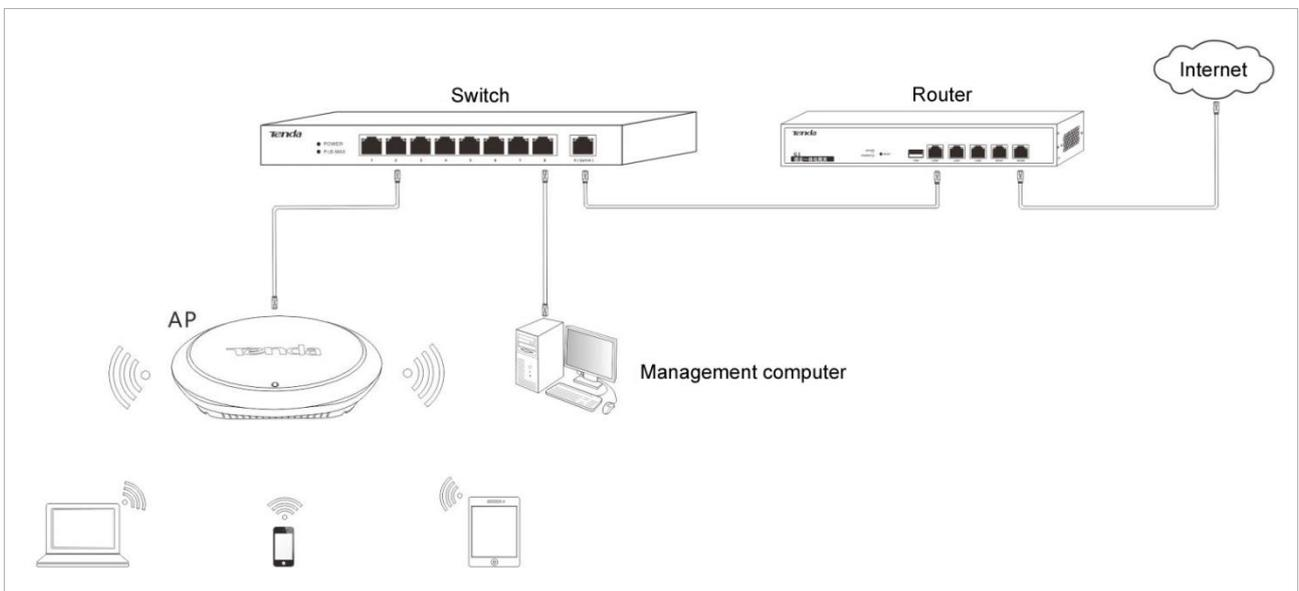
If you need to install a large number of APs, connect the APs to an M3 (Tenda AC) using the following topology so that you can manage all the APs in a centralized manner.
