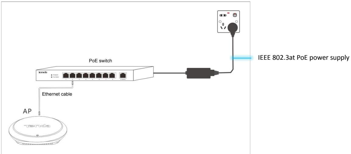
After the AP is connected to a power supply, it initializes. During initialization, the LED indicator turns solid on for 5 to 7 seconds, and then blinks. When the indicator blinks, the AP is working properly.
