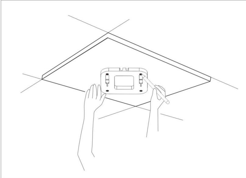
**Step 2** Create holes in the marked positions. Each hole measures at 6 mm in diameter and 25 mm to 30 mm in depth.
