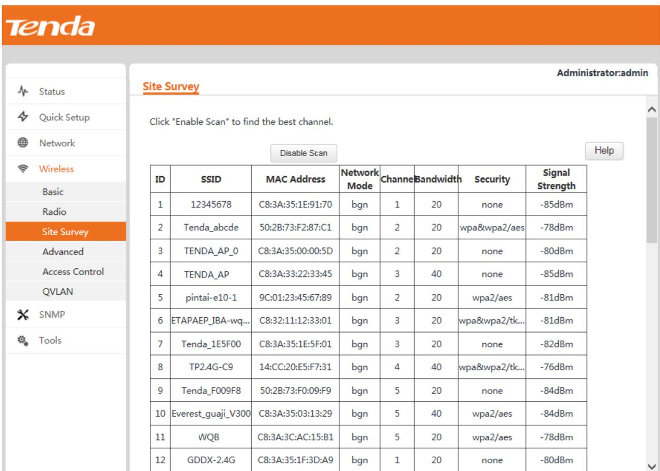
According to the scan result, you can select the least-used channel as the operating channel of the AP for better wireless transmission efficiency.
