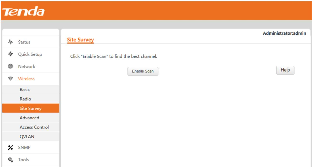
By default, the channel scan function of the AP is disabled. You can click **Enable Scan** and wait a moment for the scan result. See the following figure.
