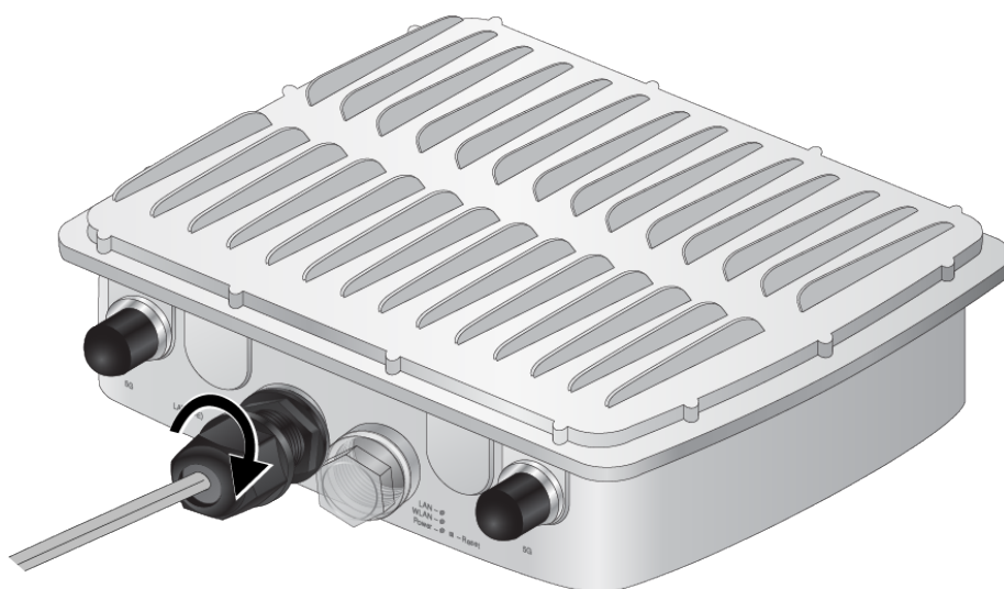
Figure 14. Tightening the Sealing Nut
