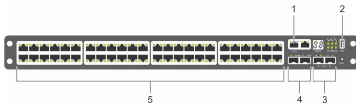
Figure 10. N3048 with 48 10/100/1000BASE-T Ports—I/O-Side
