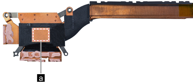
Figure 11. Areas on the heat sink where thermal interface materials should be applied
