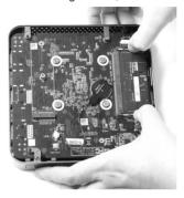
2. Remove the memory module from the slot at a 45-degree angle.
