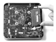
Gently press down on the memory module until it locks into place by the arms of the memory slot.
