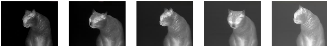
Figure 3-3 Adjust Brightness in White Hot Mode
