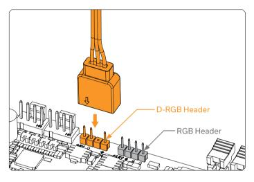
Plug the 3-pin connector from the water block's D-RGB LED light in the D-RGB HEADER on the motherboard. The LED will work if the pin layout on the header is as follows: +5V, Digital.
