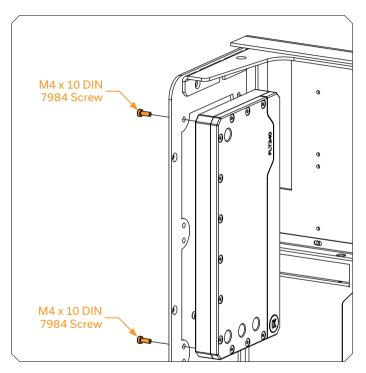
Using the included M4 screws you can mount the reservoir directly to your chassis or any other standard fan mounting location.
