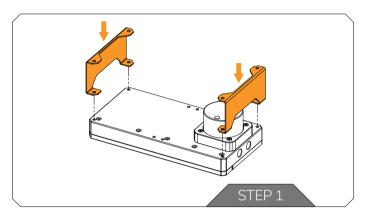
To enable installation of the reservoir onto fans, radiators or where clearance for the pump is required EK supplies a pair of FLT mounts along with M4 nuts, washers and additional screws. They can be positioned across any pair of mounting holes in several orientations.
