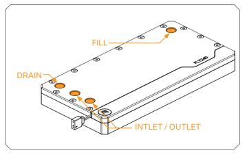
EK-Quantum Volume FLT has two ports which can be used as inlet or outlet, the chosen outlet should connect directly to your pump! The reservoir should be positioned above the pump to ensure it does not run without coolant. Both unused ports should be blocked using G1/4 plugs.
