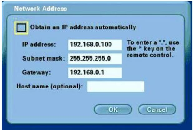
If you know you cannot be assigned an IP Address automatically through a DHCP server, then uncheck the checkbox and enter your **IP Address**, **Subnet mask** and **Gateway**.
