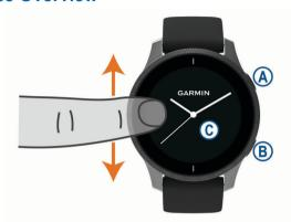
(A) Action button: Press to turn on the device.
