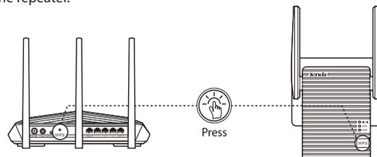
2. Wait until the Signal LED on the repeater turns solid blue or red. If not, try **Method 1**.
