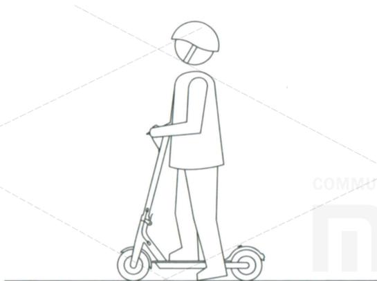
Only when both feet stand on the scooter platform, you can press the speed knob (press the knob at minimum possible scooter speed of 5km/h);
