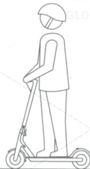
3. When it's necessary to turn, slightly move a body's center of gravity in the right direction, and turn the steering wheel slowly.
