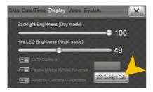
Under "LED Backlight Color" you can adjust the color of the Key illumination.
