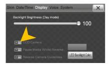
The checkbox "CCD Camera", enables the optional rear view camera function. As soon as reverse gear is engaged, the transmission of the video camera is automatically displayed on the screen.
