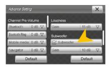
Under "Subwoofer" you can turn on or off the sound output of the RCA output SUBWOOFER and you are able to set its level from -12dB to +10db.
