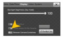
With the checkbox "Pause Media Whilst Reverse", the media playback will be paused when the reverse gear is engaged.
