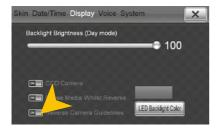
Under "Reverse Camera Guidelines" you can turn passive guidelines on or off. If the function is turned on, additional settings of the rear view camera can be made when the reverse gear has been engaged.
