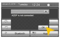
If the message "A2DP is not connected" appears, your BT device it is not connected or the audio playback is not (yet) enabled. Check the Bluetooth device and if the appropriate settings for the audio streaming are correct. Then, disconnect the device and connect it again. If the message "A2DP is not connected" appears again, the Bluetooth device does not support the A2DP standard.
