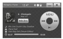
Connect your iPod<sup>™</sup> or iPhone<sup>™</sup> via USB with the ESX device. When the iPod<sup>™</sup> icon is highlighted in white (top next to the time display), the connection is active.
