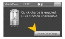
Tap on "Enable Quick Charge" to activate the quick charge function. To disable the feature again, tap on "Disable Quick Charge" at the same place position.
