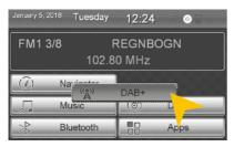
To change the position of a control panel, press and hold for 5 seconds the regarding panel in the main or apps menu until the dashed lines are visible.
