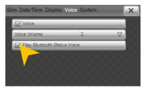
If "Play Bluetooth Status Voice" is activated, an audible confirmation of the Bluetooth<sup>™</sup> connection is issued whenever you connect or disconnect a paired Bluetooth<sup>™</sup> device.
