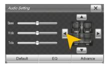
Tap on one of the seating positions or on the arrows to align the front and rear speakers.
