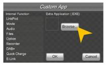
You have also the possibility to link a control panel with any compatible software application (. EXE), which must be stored on the available storage locations. Tap on "Browse" to select the desired application.
