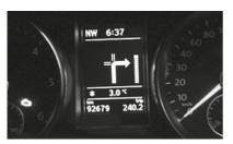
The multi-function display (MFA) between the speedometer displays will also be supported by the device and displays e.g. the directional arrows from the ESX Navisoftware and RDS information of the radio.
