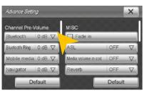
On the left under "Channel Pre-Volume" you can set the individual volume for each application. Just tap on the arrow icons to change the value upward or downward.
