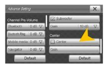
Unter "Center" you can turn on or off the sound output of the RCA output CENTER and you are able to set its level from -12dB to + 10db.
