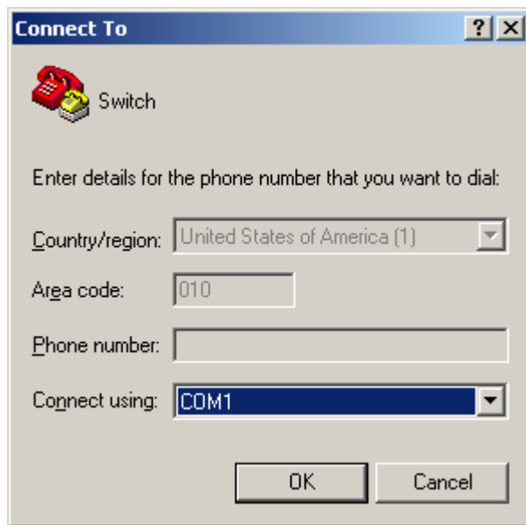
Figure 9 Setting the serial port used by the HyperTerminal connection
