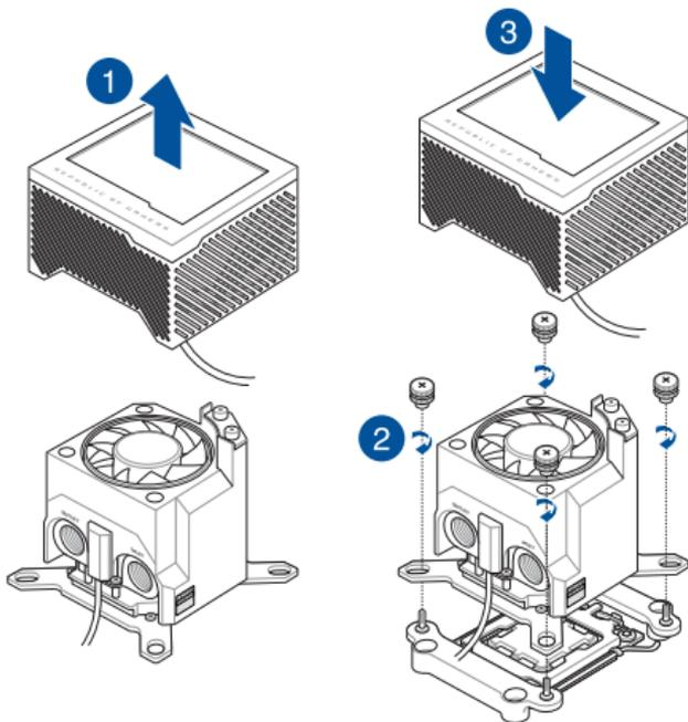
**NOTE:** We recommend installing the water block so that the ports of the water block face towards you for optimal performance (motherboard positioned with rear IO ports on your left).
