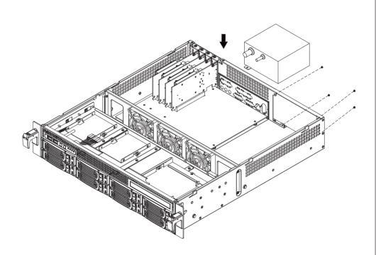
4-2 If installing 2U single or redundant power supply, attach corresponding power supply plate to the chassis first, then place the power supply into the chassis and secure with screws
