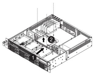
5-2 Install optical drive into the bracket, secure with screws and reinstall the assembled drive bracket back into the chassis
