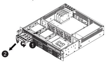
7-2 Install drive into the drive tray, secure with screws and reinsert the assembled drive tray back into the chassis
