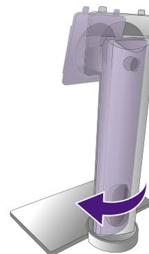
Tighten the thumbscrew on the bottom of the monitor base as illustrated. And then turn the stand counterclockwise to face forward.
