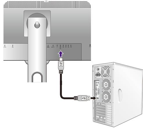
Connect USB devices via other USB ports (downstream) on the monitor. These downstream USB ports transmit data between connected USB devices and the upstream port.
