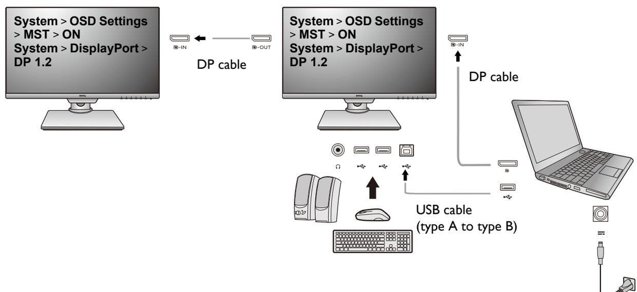
1. Set the monitor ready for connection. On the monitor, go to **System > OSD Settings > MST**, and select **ON**. Go to **System > DisplayPort**, and select **DP 1.2**. Note the OSD menu can be launched and configured only when input signal is detected.
