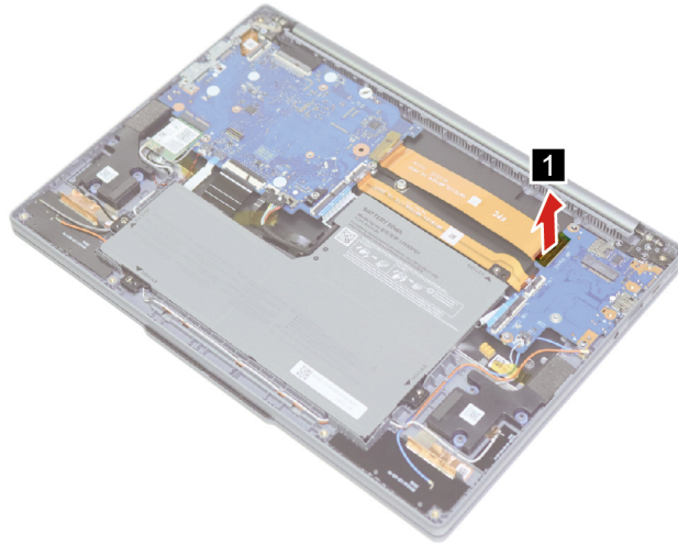
Figure 14. Peel off the right tape of the 36-pin I/O board cable
