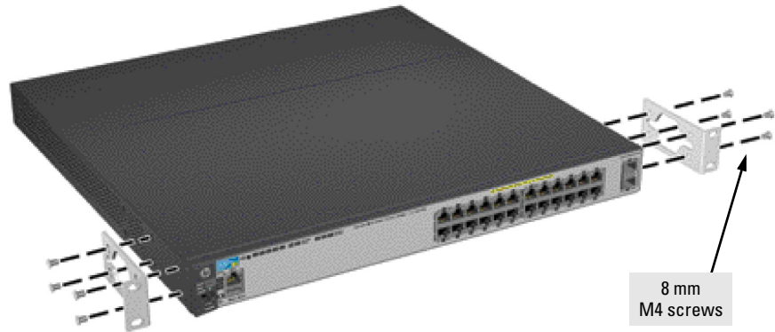
Figure 2-9. Attaching the mounting brackets to the switch
