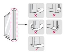
When holding the monitor, the screen should face away from you to prevent it being scratched.
