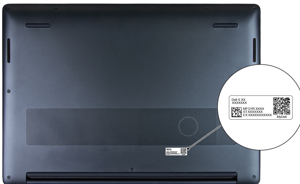
Figure 6. Service Tag/Express Service Code location
