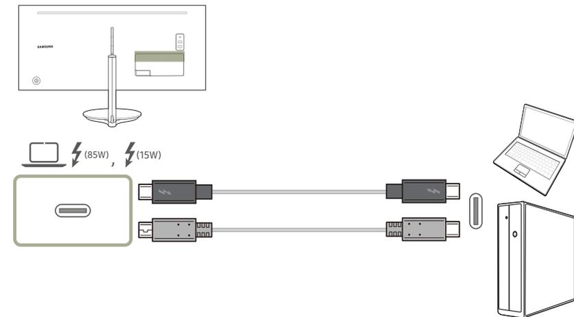
Connect the Thunderbolt™ 3 cable or USB Type-C cable to
