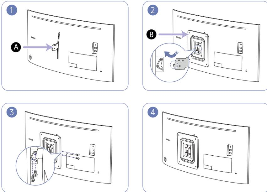
**A** Attach the Wall-mount bracket here
