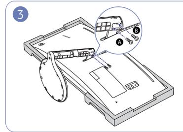
Rotate **A** and **B** screws for fixing.
