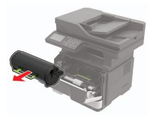
**3** Remove the used imaging unit.
