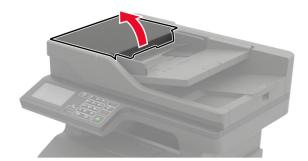
**2** Remove the used ADF separator roller.
