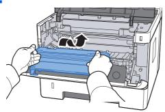
**13** Return the developer unit together with the toner container to its position, aligning the guides at both ends with the slots in the machine.
