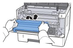
**9** Return the developer unit together with the toner container to its position, aligning the guides at both ends with the slots in the machine.
