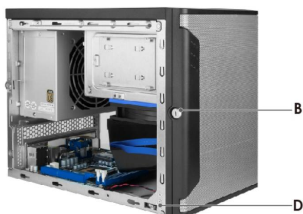
Figure 5 Padlock Loop and intrusion switch location
