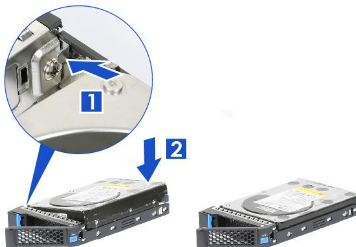
Figure 12 3.5" HDD installation (tool-less type)
