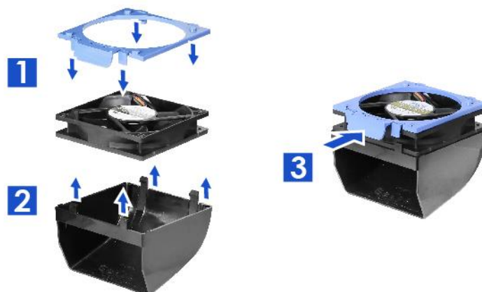
Figure 16 HDD fan installation (fan assembly)
