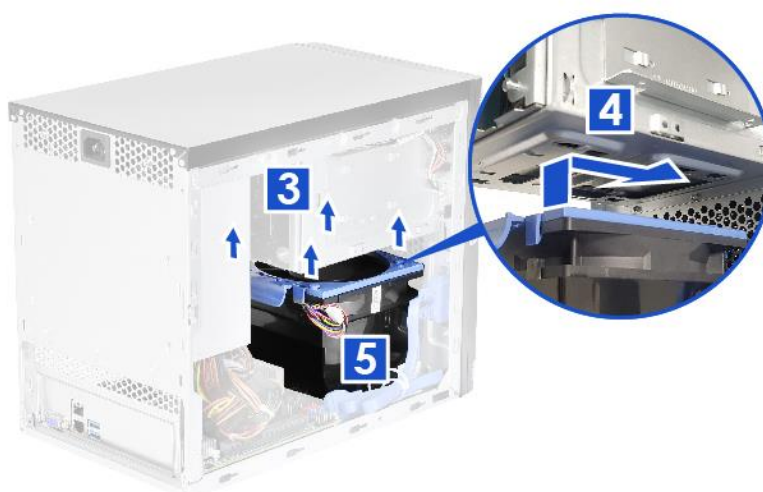
Figure 17 HDD fan installation (chassis)
