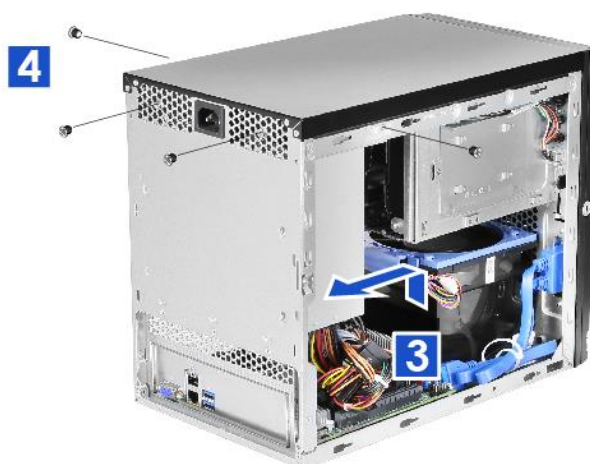
Figure 20 Single PSU installation-2
