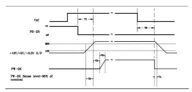
Figure 2. PS-OK Timing Sequence
