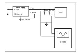
Figure 1. Ripple/Noise voltage test circuit
