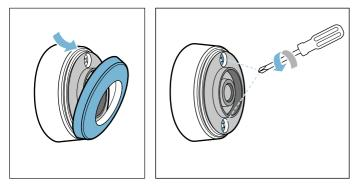
2. Remove the upper section of the casing. Take the old batteries out. Put the new batteries in. Make sure that the polarity is correct.
