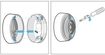
4. Put the silicone cover back on the lower section of the temperature sensor casing.
