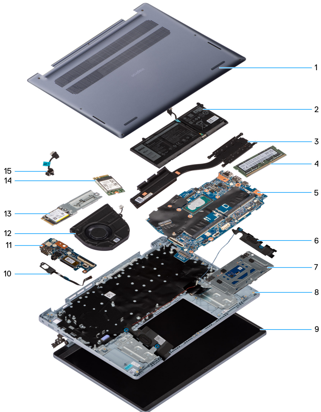
Figure 10. Major components for computers that are shipped with an aluminum chassis
