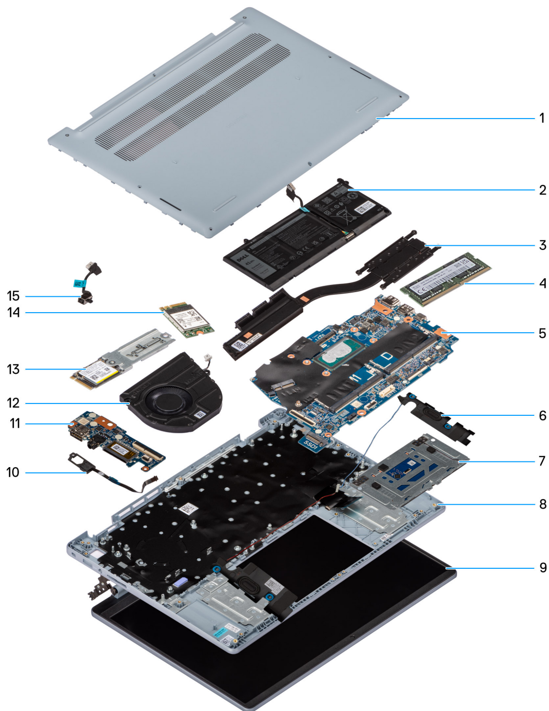
Figure 9. Major components for computers that are shipped with a plastic chassis
