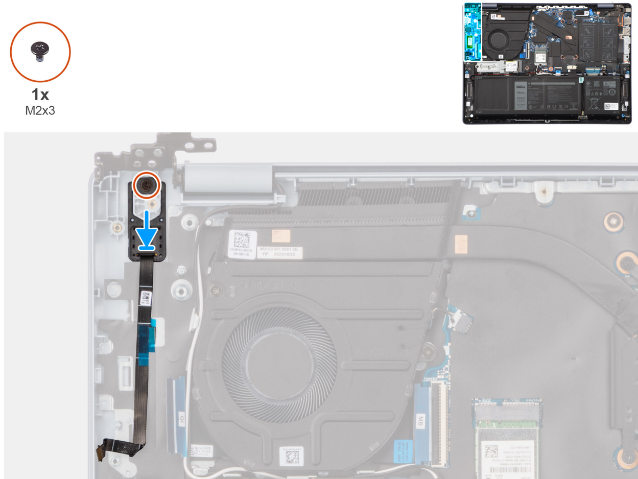
Figure 59. Installing the power-button with fingerprint reader
