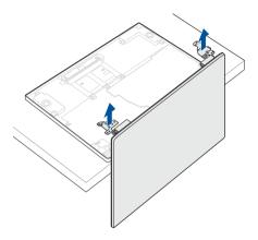
1. In the orientation shown, align and place the hinges of the display panel module on the screw holes.
