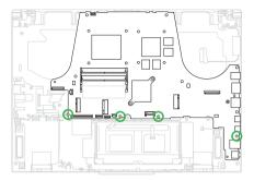
1. Align and install the motherboard, then secure the motherboard using the screw(s) you removed earlier.
