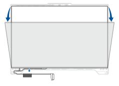
4. Disconnect the cable from the rear side of the display panel.
