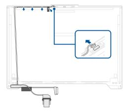
3. Carefully remove the camera module, then remove the rubber caps from the camera module.
