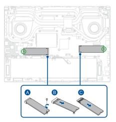
4. Remove the absorber sheet(s) from the M.2 SSD module(s).
