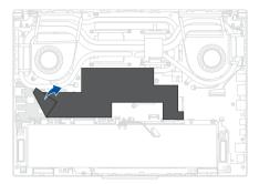
2. Peel off the aluminum foil (if available) from the top RAM module slot and remove the foil.
