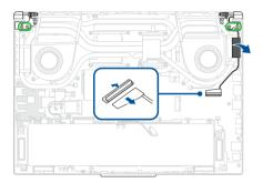
4. Remove the display panel module.
