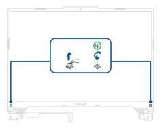
3. Carefully pry the bezel loose from the bottom left corner, then remove the bezel completely.
