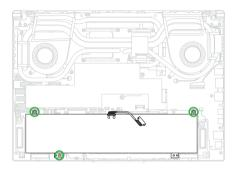
4. Remove the battery power cable.
