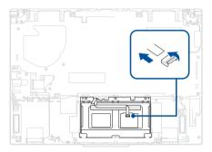
2. Remove the screw(s), then remove the touchpad module.
