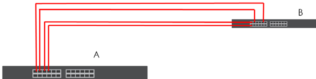
Figure 125 Trunking Example - Physical Connections
