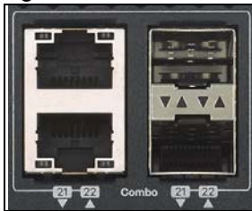
Figure 14 Combo Port Example: 10 Gigabit Port and SFP+ Transceiver Slot
