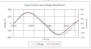
Input AC Current Waveform (ITHD = 8.08%, 50% Load)
