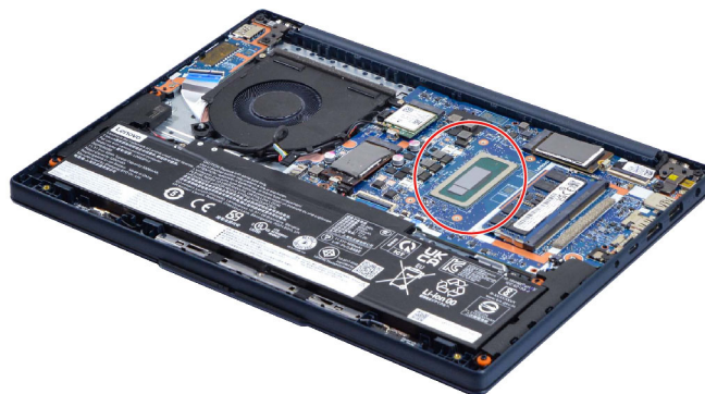
Figure 22. Areas on the system board where thermal interface materials are applied
