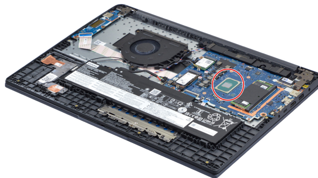
Figure 67. Areas on the system board where thermal interface materials are applied
