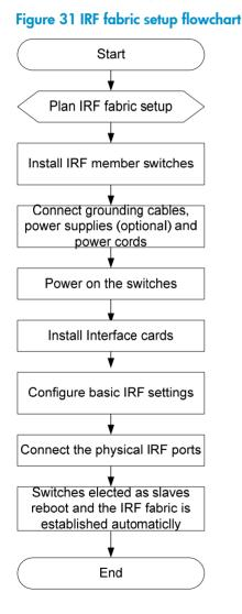
To set up an IRF fabric:
