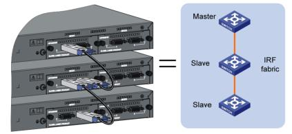
Figure 33 IRF fabric in ring topology
