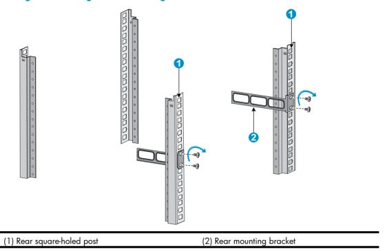
Figure 7 Attaching the rear mounting brackets to a rack
