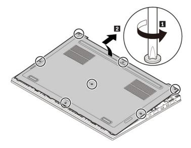
5. Install the new bottom cover as shown and tighten the screws.
