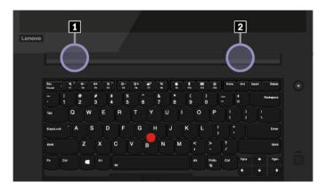
■ Wireless-LAN antenna (auxiliary)■ Wireless-LAN antenna (main)
