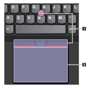
By default, both the TrackPoint pointing device and the trackpad are active with the touch gestures enabled. To change the settings, see "Customizing the ThinkPad pointing device" on page 21.
