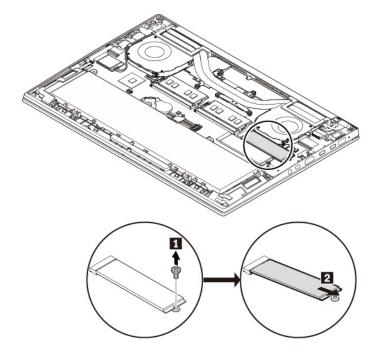
6. Align the contact edge of the new M.2 solid-state drive with the key in the slot. Then carefully insert the new M.2 solid-state drive into the slot at an angle of about 20 degrees. Pivot the M.2 solid-state drive downward and install the screw.
