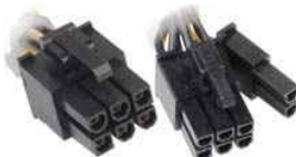
Additional power plugs for graphics cards with 6 and 6+2 pins
