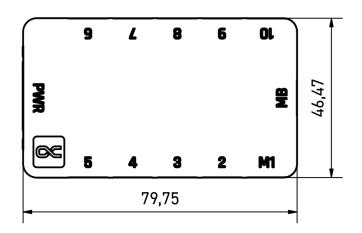
General tolerance: ± 0,25mm Dimension in millimeter
