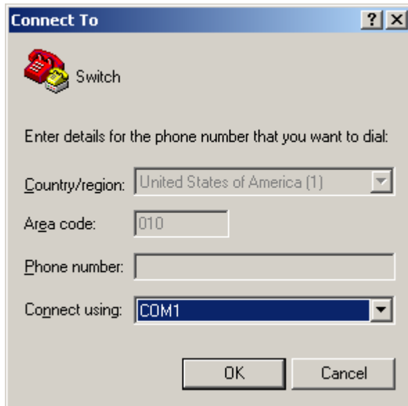
Figure 32 Set the serial port used by the HyperTerminal connection
